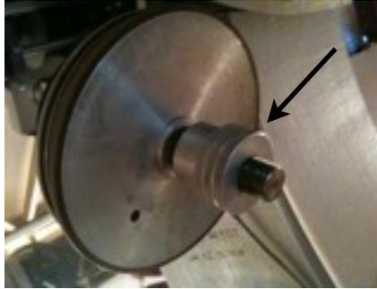
*Picture 1: R.A. Clutch Adjustment Knob*
